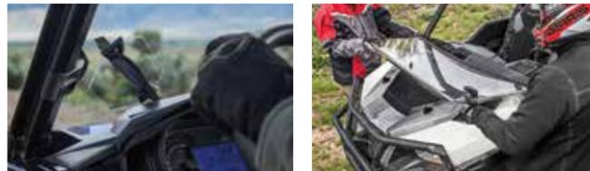
Offers fully-sealed or flipped-down venting options. Upper half detaches, leaving lower half for protection with maximum ventilation.
